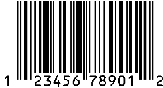
Figure 25 Quiet Zone in a Bar Code
