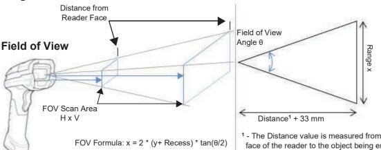
Note: The Recess value of 33 mm is the distance from the reader front face to the image sensor inside the reader. The **Distance and Recess** values are added together for the FOV Scan Area calculation.
